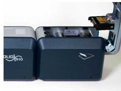
Figure 23 Installing the film cartridge
