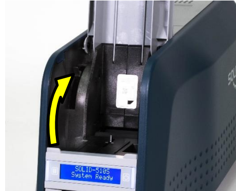
Figure 24 Adjusting the card thickness lever
