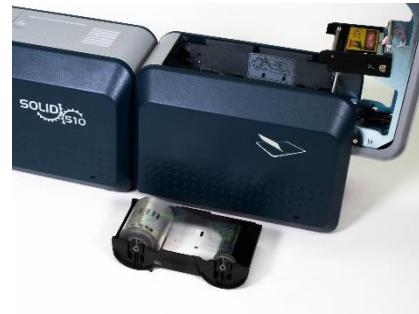
Figure 22 Loading the laminating film
