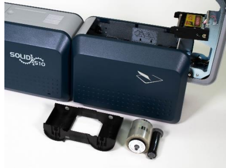
Figure 21 Take out the film cartridge
