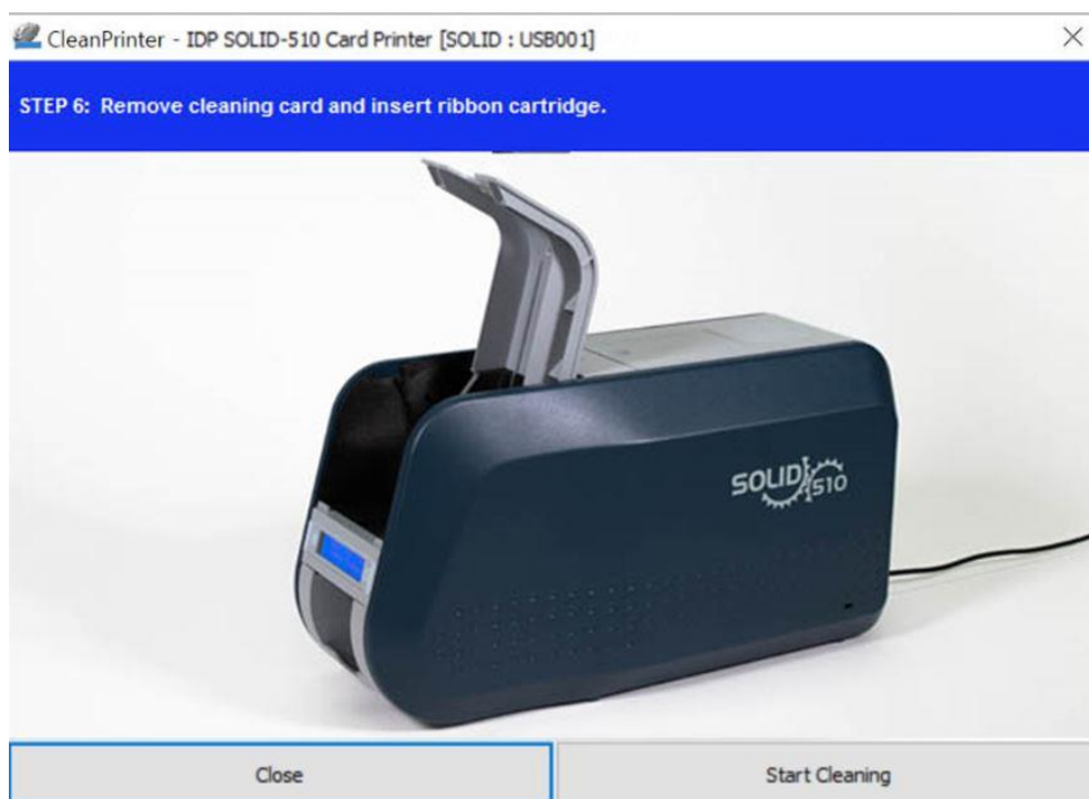
Figure 111 Printer cleaning Step 6
